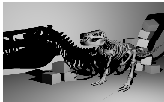
Figure 16: Irregular Z-Buffer sample frame: this method uses an irregular spatial data structure to produce alias-free shadowing. Like the transparency example in figure 15, the data structure is tightly integrated with the rendering pipeline. The renderer constructs the shadowmap and then treats it as a special class of frame buffer. (Skeleton model by TurboSquid.)
