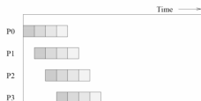
(c) The same message broken into four parts and sent over the network.
