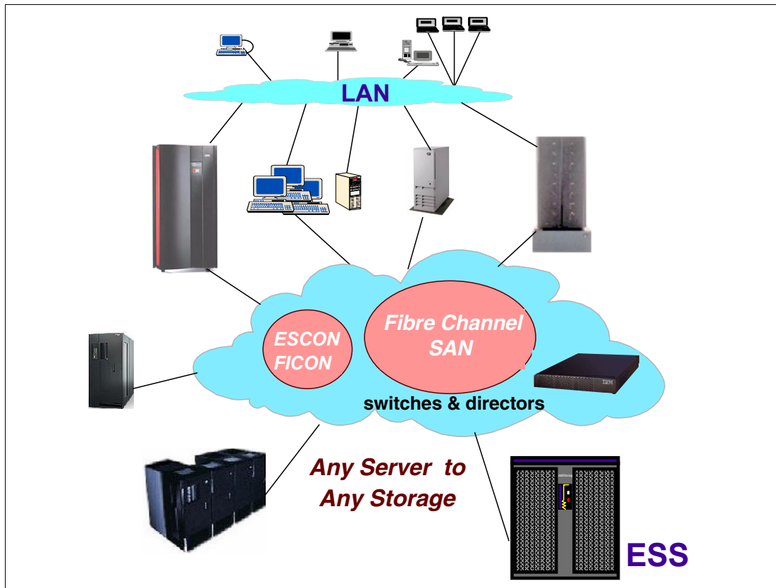
Figure 3-28 Storage area network (SAN)
