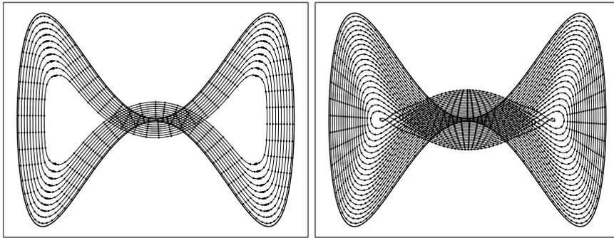
FIGURE 1. Isotropic curvature driven motion,  $\beta(k, \nu) = \varepsilon k + F$ , with  $\varepsilon = 1$ ,  $F = 10$ , without (left) and with (right) uniform tangential redistribution of grid points.
