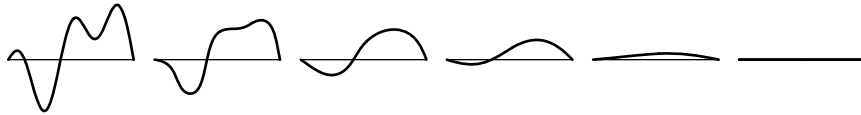
Figure 4: Evolution of a graph y = u(x, t) by the curvature flow equation u_t = \frac{u_{xx}}{1 + u_x^2} ( 0 < x < 1 ) (from left to right). The boundary condition is u(0) = u(1) = 0 , and the initial curve is given by u(x, 0) = 0.1 \sin(\pi x) - 0.3 \sin(2\pi x) + 0.2 \sin(5\pi x) .
